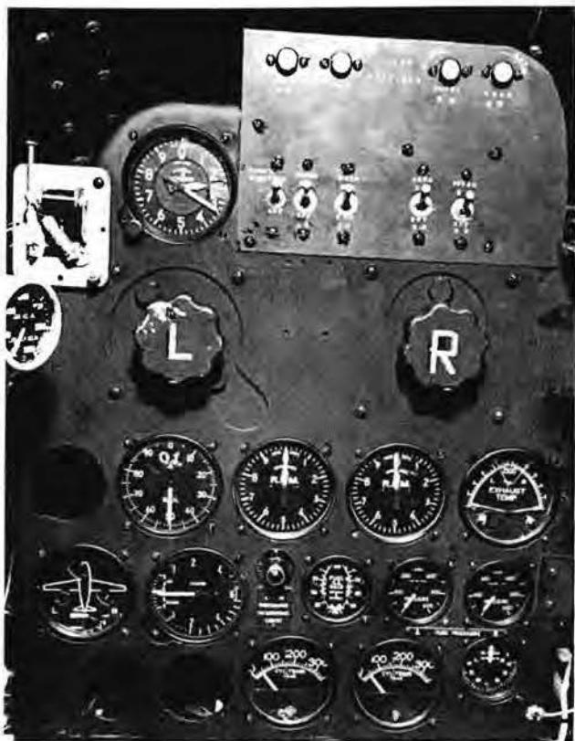
Doorbell mechanism on the instrument panel can be seen in the upper right corner of this image. The "cyl temp" gauges (at bottom) were actually used to display engine bearing temperatures.
