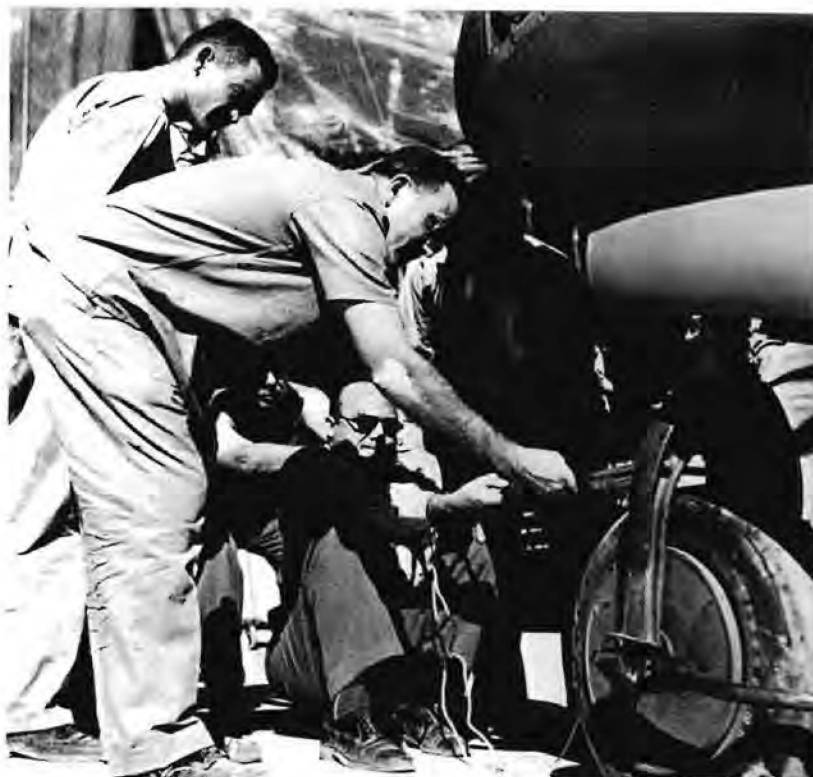
D. Roy Shoults (seated) checking the spring scale that measured installed engine thrust. Bob Stanley (at left) and Bell onsite test manager Ed Rhodes (foreground) look on.
