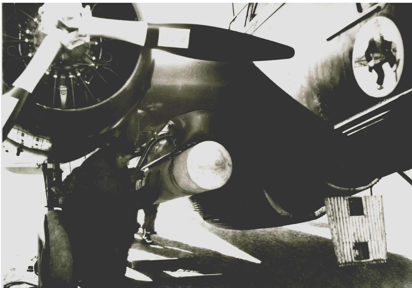
Above: a large concrete bomb-shape is loaded onto a B-12 for training use. Over the course of the Range's life, the detachment used bombs up to 2,000 pounds.
