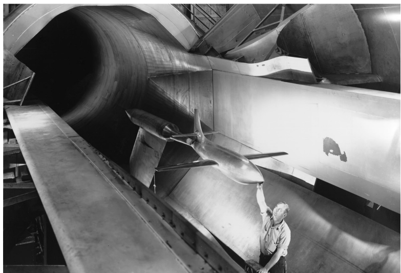
Above: Front and rear views of the XS-1 which illustrate its bullet-like shape, the arrangement of its flight controls and the relatively small size of the exhaust nozzles for each of the chambers of its 6,000-pound thrust engine. Below: Model of the XS-1 in the Langley Memorial Aeronautical Laboratory high-speed wind tunnel.
